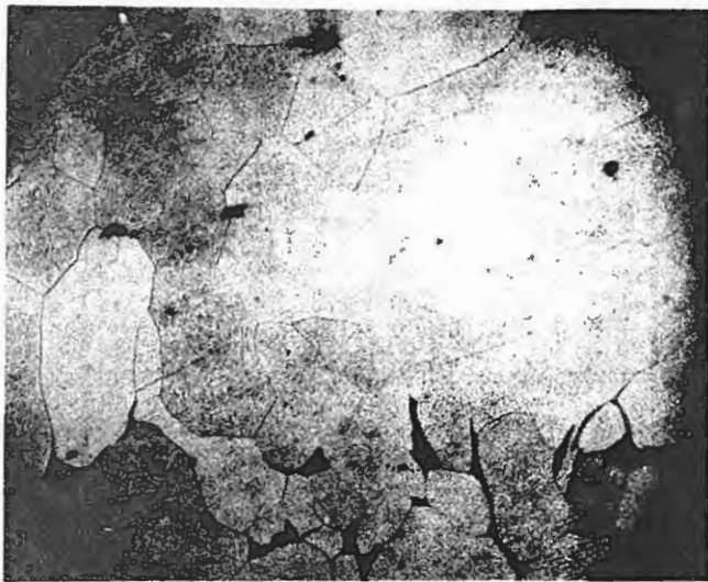
Figure 32. Structure of Japanese wrought iron, Hocho Tetsu, for the core of the sword.
